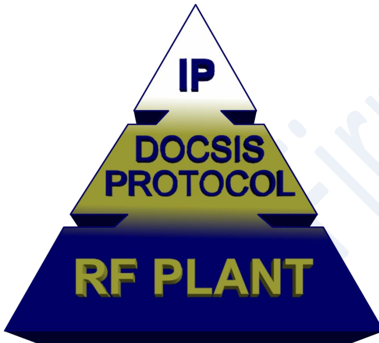
Figure 1. DOCSIS Network Functional Layers
