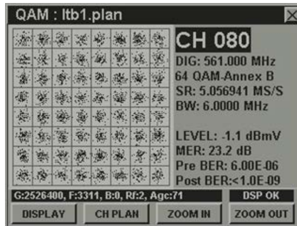
Figure I-26 - 64-QAM Signal With Poor (23.2 dB) MER
