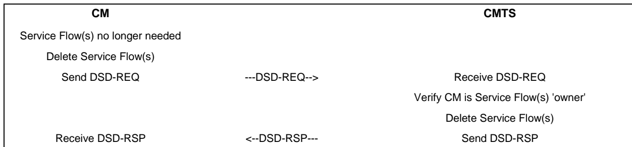
Figure 11–32 - Dynamic Service Deletion Initiated from CM
