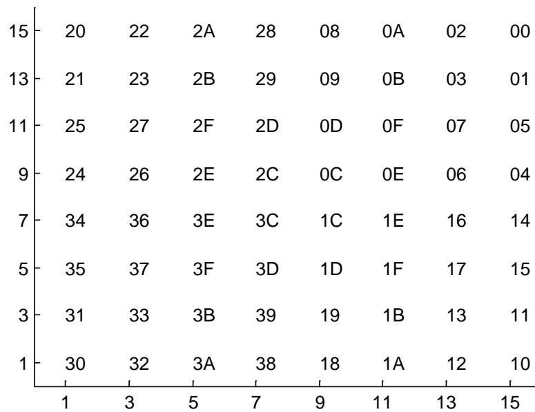
Figure A-10 - 256-QAM Constellation Mapping of \{y_2y_3y_4y_5y_6y_7\} on to Quadrant 1
