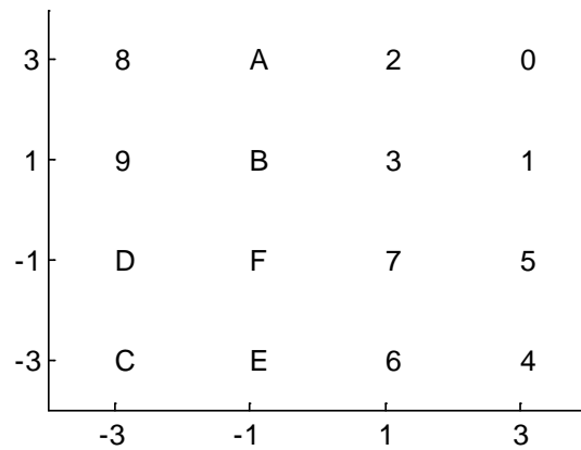
Figure 7-75 - 16QAM Constellation Mapping of \{y_{i,0} y_{i,1} y_{i,2} y_{i,3}\}
