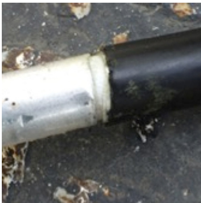
Figure 2: Trunk line outer shielding cut by technician when coring cable for connector, illustrates another common issue identified with PNM — outside plant impairments.
