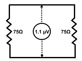
The carrier-to-noise ratio of an individual amplifier can be calculated with the formula
