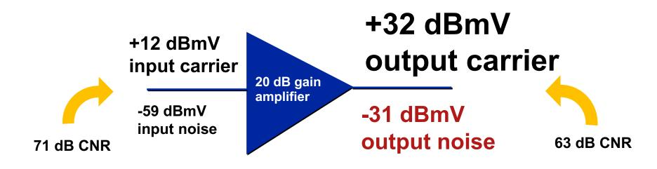
In this example, the output CNR is worse than the input CNR by 8 dB! The degradation of the carrier-to-noise ratio through the amplifier is called the amplifier's **noise figure**. Don't worry, you don't have to calculate noise figure. Amplifier manufacturers publish noise figure in their product specifications.
