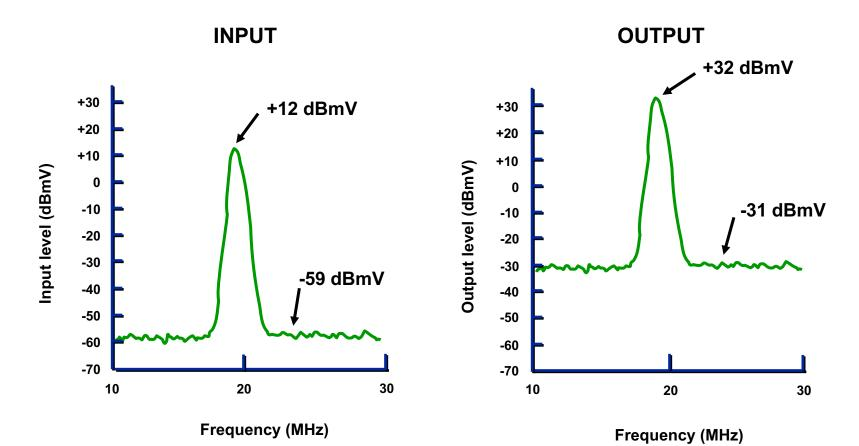
The noise level at the amplifier output has increased more than the carrier level because of added noise from amplifier circuits.
