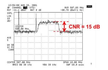
For SC-QAM CNR measurements, a noise floor correction is not necessary. (Just make sure the displayed noise is not test equipment noise.)
