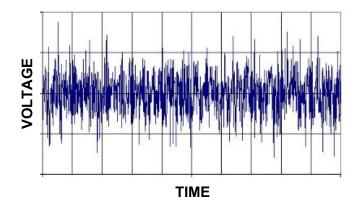
According to a Hewlett-Packard application note\* on noise figure measurement, thermal noise is defined as "the fluctuating voltage across a resistance due to the random motion of free charge caused by thermal agitation."
