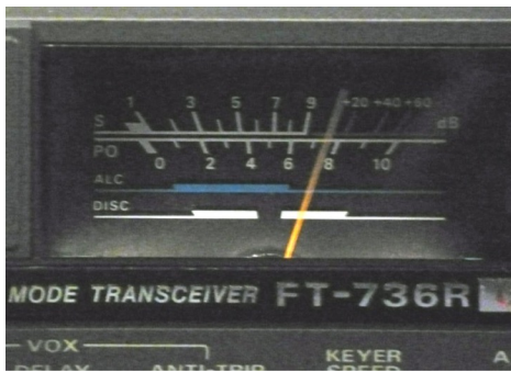
Communications transceiver's S9+15 dB S-meter reading caused by 400 \mu\text{V}/\text{m} digital leak at 10 ft.
