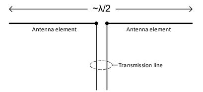
Dipoles form the basis for several other antennas, such as Yagi-Uda ("Yagi") and log periodic dipole array (LPDA) antennas.
