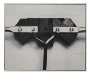
Attach the transmission line to the elements using suitable hardware. Make sure the screws are long enough to pass through the bracket. Then use a tubing cutter to trim the lengths of the elements so the endto-end dipole length is the calculated value (42 inches for this project).
