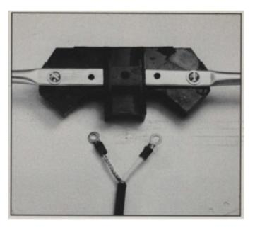
Remove about 1-1/2 inches of jacket from one end of the transmission line. Remove 1/4 inch of dielectric from the center conductor, then crimp and solder the wire terminals to the shield and center conductor.
