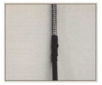
Install a short length of heat shrink tubing over the soldered (or tie-wrapped) connection, and shrink with a heat gun or blow dryer.
