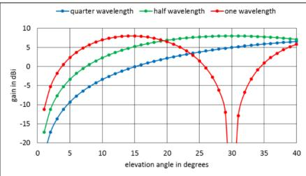
Calculated results for a 14 MHz half-wave dipole modeled over average earth conditions, for antenna heights of  $\lambda/4$ ,  $\lambda/2$ , and  $\lambda$ .
