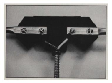
Slip a couple feet of copper shield from a piece of RG-8 coax over the antenna feedline, until the upper end of the larger shield is about flush with the end of the transmission line's coax. Secure the larger shield to the transmission line with a tie wrap, making sure the larger shield does not touch the smaller cable's exposed shield.
