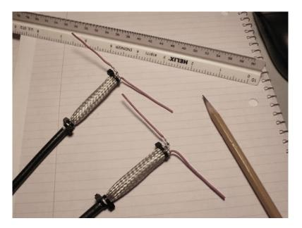
Center insulator: None Elements: Small gauge insulated wire Feedline: Series 59 copper braid coax Balun:  $\lambda/4$  sleeve balun
