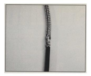
Trim the lower end of the RG-8's shield to line up with the transmission line's exposed shield. Carefully solder the larger shield to the transmission line's shield (I've sometimes used several small tie wraps to do this instead of soldering).
