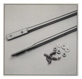
Flatten about 1-3/4 inch of one end of each of the two TV antenna elements in a bench vise. Drill two 1/8 inch holes about an inch apart in the flattened areas.
