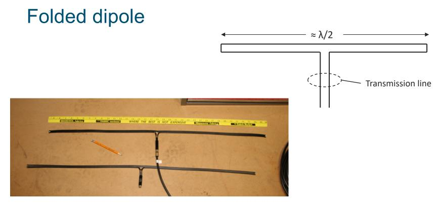
**Element:** 300 ohms twinlead, ends soldered together, fed in center of "bottom" element **Feedline:** Suitable length of Series 6 or Series 59 drop cable **Balun:** Cable TV matching transformer (300 ohms-to-75 ohms)
