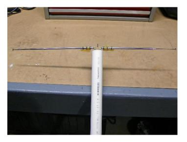
**Mast:** 1-inch PVC pipe (Sch. 40) with notches cut in top to fit center insulator; length is about 3-1/2 feet.
