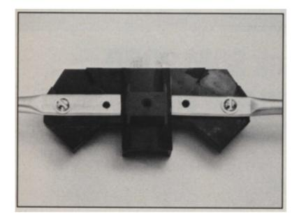
Attach the elements to the plastic bracket using only the outer holes. The inner holes will be used to attach the transmission line to the elements. For this project, a 15 ft. length of copper braid Series 59 coax was used.
