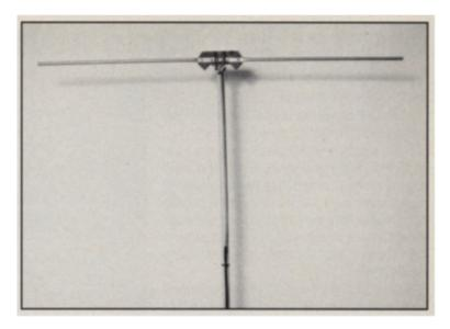
Attach the plastic bracket to the end of a wooden dowel (an old broom or mop handle will work). Tie wrap the feedline to the wooden pole in a couple places, then install an F connector on the other end of the transmission line.
