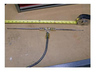
Center insulator: acrylic sheet (0.1 inch thickness) Elements: telescoping antennas Feedline: Mini 75 ohm coax, about 5 feet Balun: #43 mix ferrite beads
