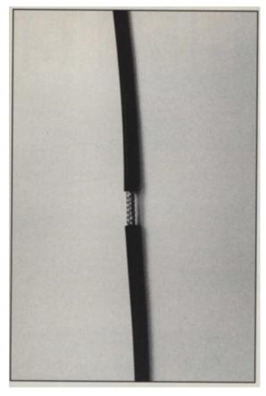
Measure about 21 inches down from the top end of the coax (from the end of the jacket where the center conductor and shield separate). Carefully remove about 3/4 inch of jacket from the coax.
