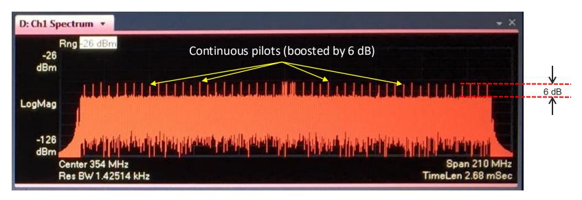
Continuous pilots always remain on the same frequencies, and are configured to be spread more or less uniformly throughout the OFDM channel. Another type of pilot called scattered pilots – which are also boosted by 6 dB – are not shown here (they change frequency throughout the OFDM channel).
