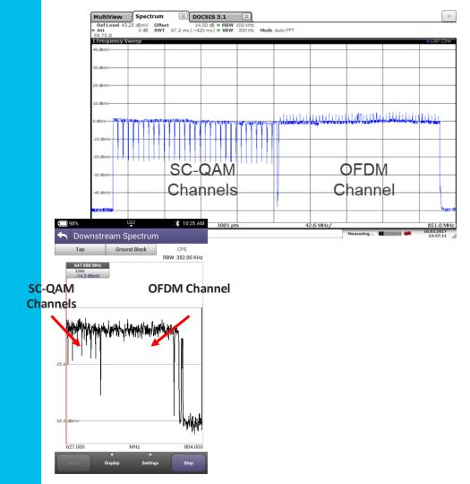
The test equipment must be locked to the PLC. If lock to the PLC cannot be achieved, then DOCSIS 3.1 operation won't be possible.
