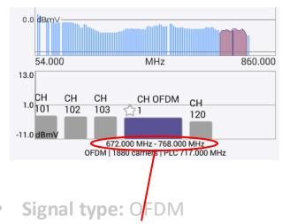
• Channel bandwidth: 672 MHz to 768 MHz (96 MHz)
