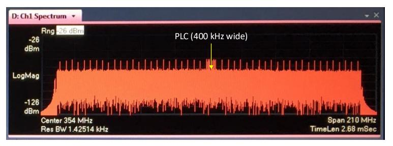
The PLC, which is 400 kHz wide and is centered in the 6 MHz-wide PLC band, comprises eight subcarriers (50 kHz spacing) or 16 subcarriers (25 kHz spacing), each using 16-QAM to convey physical layer parameters to the cable modems.
