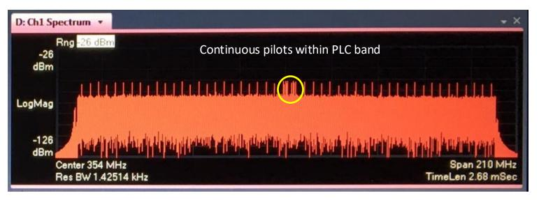
The continuous pilots in the PLC band have a unique pattern that tells the modem where the PLC is located. This pilot pattern is not user-adjustable; it is a fixed pattern defined in the DOCSIS 3.1 PHY Specification.
