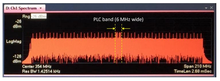
The PLC band is a 6 MHz-wide portion of the OFDM channel within which the PLC is centered. The PLC band cannot have any excluded subcarriers or exclusion bands.
