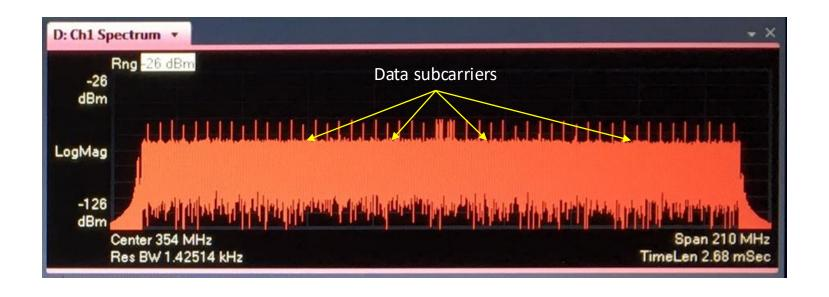
Active subcarriers in a 192 MHz-wide channel: 7600 subcarriers with 25 kHz spacing (called "8K FFT") or 3800 subcarriers with 50 kHz spacing (called "4K FFT")
