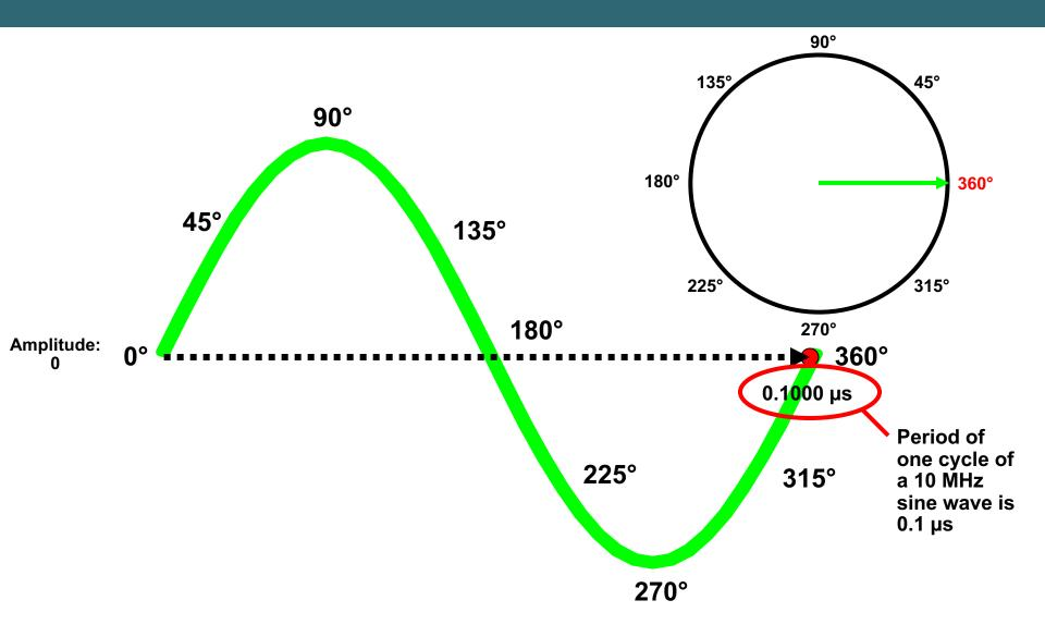
Knowing that one wavelength (cycle) of a sine wave equals 360 degrees of phase, we can now figure out the total number of degrees of phase the 100 ft piece of cable represents at each frequency
