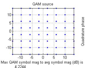
Base-band complex waveform peak to RMS(dB) is 7.9459
